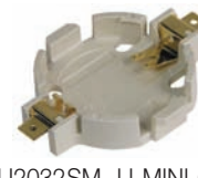
BU2032SM-JJ-MINI-GTR recessed into pcb
